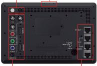
SDI, HDMI, YPbPr, Ethernet, GPI(RJ45), S-Video, CVBS RS444
