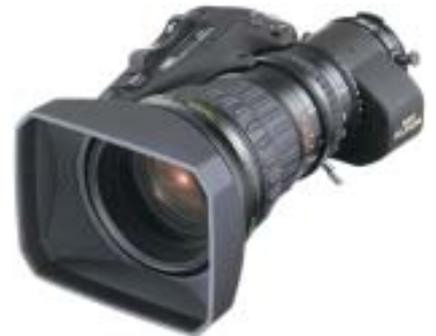
With the longest focal length, 137 mm (274 mm with 2X Extender), and the widest angle of view (64° 30') at 7.6 mm, the HA18x7.6 is the new HD standard lens for all high-definition broadcast news and field production applications in 16:9 image format.
