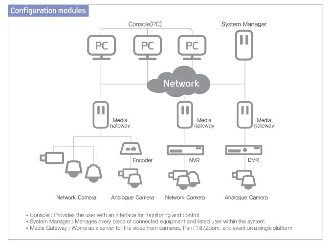
Up to 5 clients can simultaneously access the server that manages and monitors the remote devices with real-time access to the video sources, providing efficient/effective monitoring solution.
