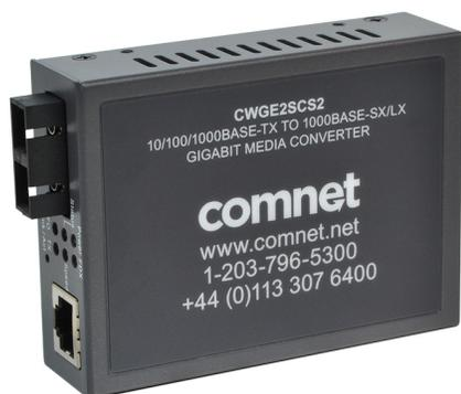
The ComNet™ CWGE2SC(M,S)2 Ethernet media converters are designed to transmit and receive 10/100/1000 Mbps data over multimode or single mode optical fiber. The electrical interface will Auto-Negotiate to a 10, 100, or 1000 Mbps Ethernet rate without any adjustments. The optical interface operates at a 1000 Mbps Ethernet rate. These media converters are commercial grade for light industrial use.
