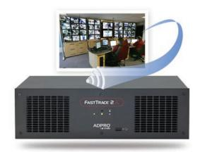
The ADPRO FastTrace 2E is the best-in-class video recording and alarm transmission solution available. This hardware platform now runs the latest ADPRO XO Security Operating System, to create a powerful Remotely Managed Multiservice Gateway (RMG). The RMG is scalable up to 32 video channels, of which 4 to 20 analogue channels, expandable with up to 32 IP channels. Furthermore, up to 32 analytic channels are possible.
