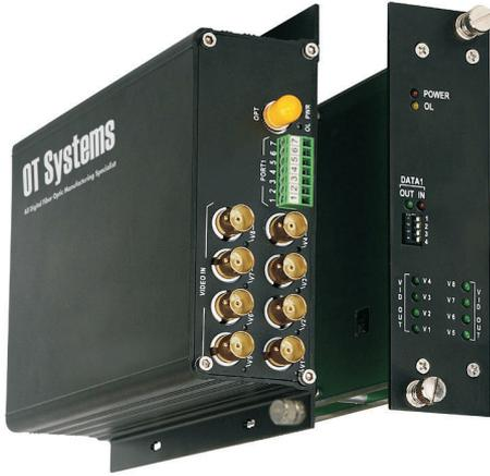
The FT8X0DB series supports optical transmission of high-quality 10-bit PCM coded video with bi-directional data through one fiber either in multimode or singlemode.
