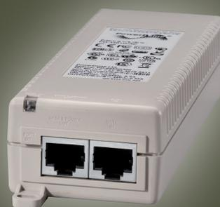
The SNCA-POE1 PoE midspan offers a cost effective, fully IEEE 802.3af compliant solution to power edge-based IP cameras and other Ethernet devices with PoE, providing a maximum of 15.4 watts of power and ensuring safe operation of any IEEE standard IP camera. The SNCA-POE1 provides PoE to IP security cameras and other Ethernet-based devices to receive power, along with data, over standard Ethernet cables, leaving network infrastructure completely unaltered.
