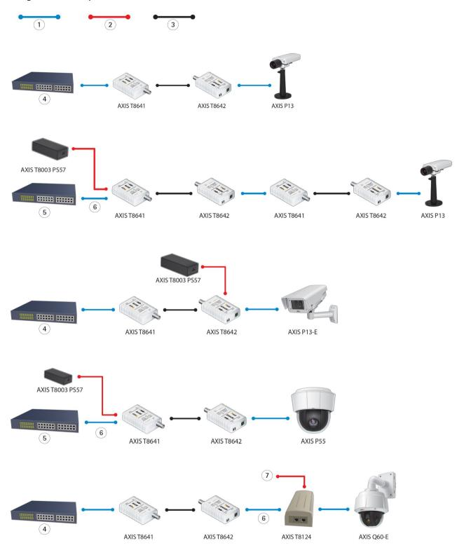
[1] Power and Data over Ethernet, [2] Power, [3] Power and Data over Coax, [4] PoE Switch, [5] Ethernet Switch, [6] Data only, [7] AC Power
