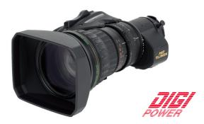
With a long focal length, 137 mm (274 mm with 2x Extender), and a wide angle of view (64° 30') at 7.6 mm, the HA18x7.6 is the HD standard lens for all High Definition broadcast news and field production applications in 16:9 image format.
