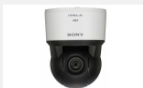
SNC-ER550 Rapid-Dome-Kamera, 720p/30 Bilder/s – E-Serie
