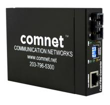
The ComNet™ CWFE2SC(M,S)2 Ethernet media converters are designed to transmit and receive 10/100 Mbps data over multimode or single mode optical fiber. The electrical interface will Auto-Negotiate to a 10 Mbps, or 100 Mbps Ethernet rate without any adjustments. The optical interface operates at a 100 Mbps Ethernet rate. These media converters are commercial grade for light industrial use.
