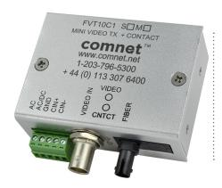
The ComNet™ FVT10C1(M,S)1/M series video transmitters transmit one channel of video plus one contact closure over one optical fiber. The FVT10C1M transmitter is available in multimode and single-mode versions.
