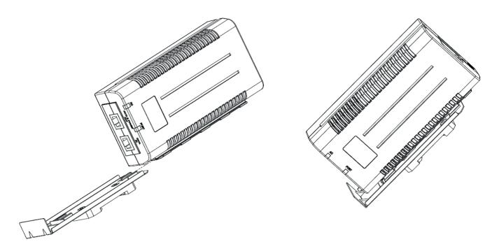
Assemble AXIS Midspan DIN Clip A onto the midspan and mount it upwards along the DIN rail.
