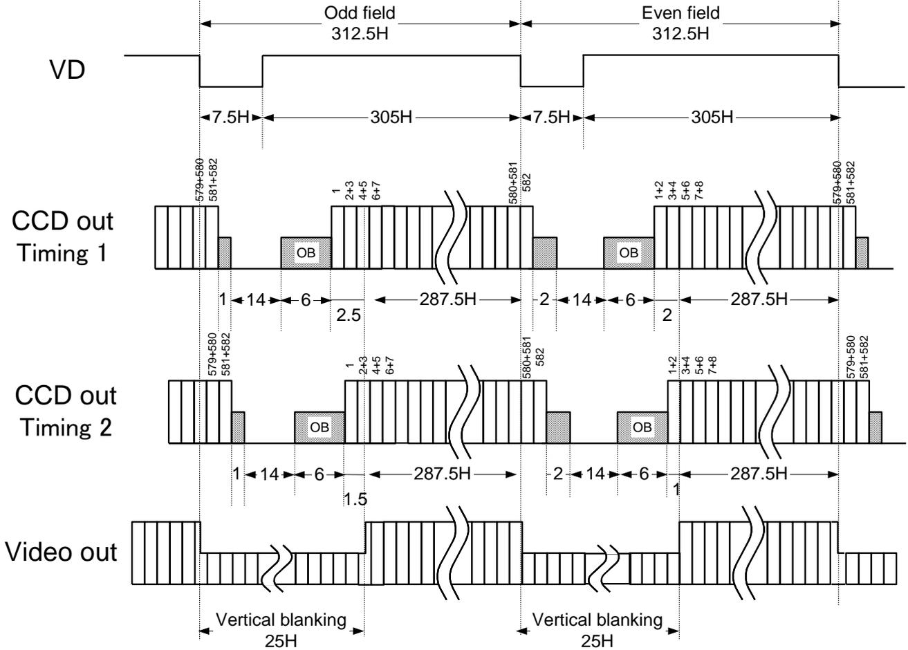
\* CCD out timing 1 DIP-SW5 = OFF state, CCD out timing 2 of DIP-SW5 = ON state
