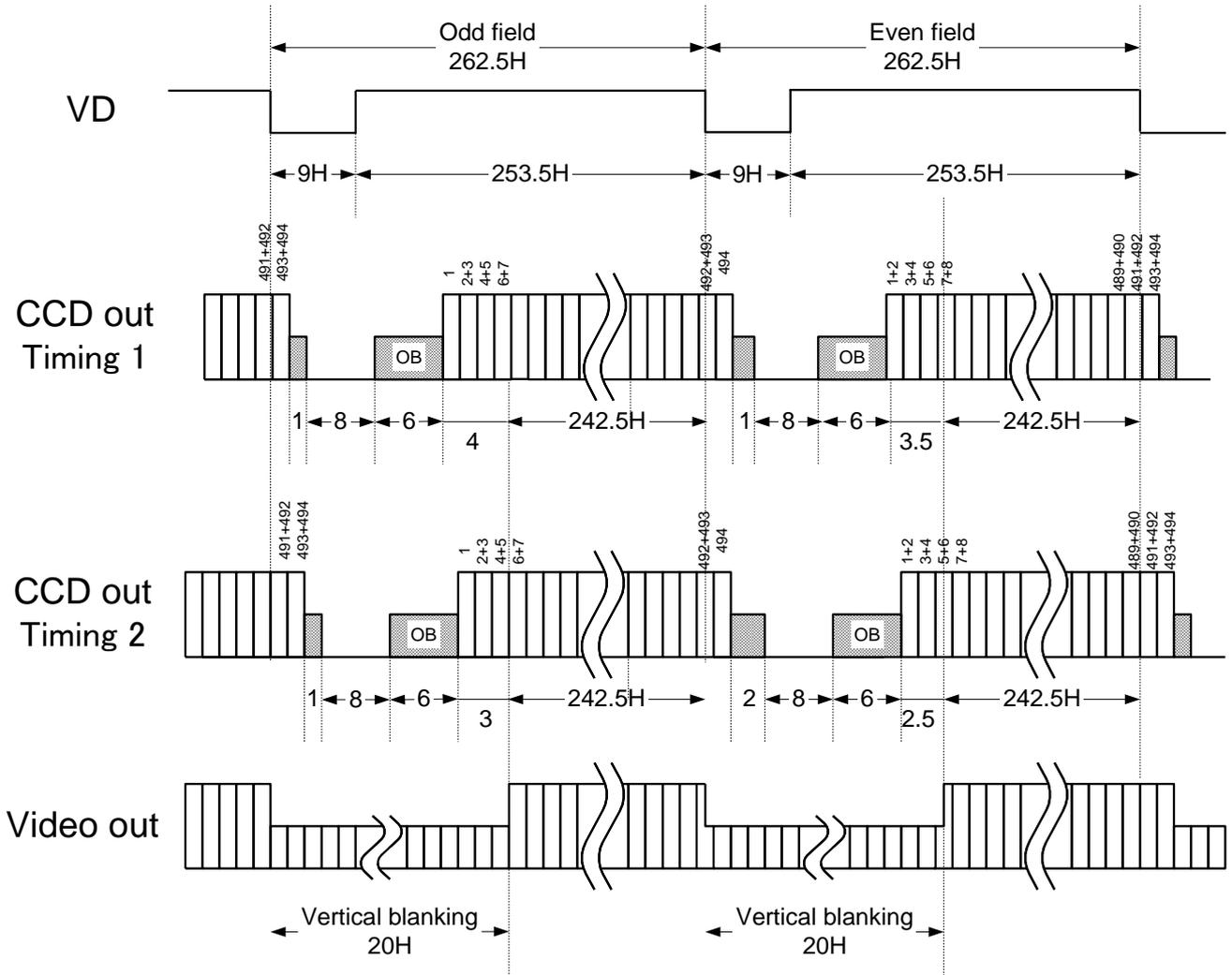
\* CCD out timing 1 DIP-SW5 = OFF state, CCD out timing 2 of DIP-SW5 = ON state
