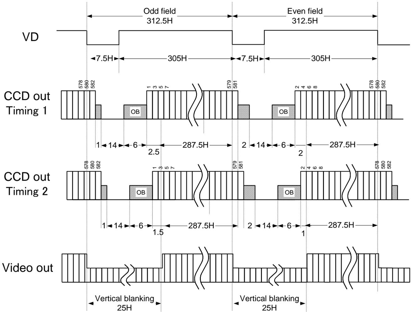
\* CCD out timing 1 DIP-SW5 = OFF state, CCD out timing 2 of DIP-SW5 = ON state
