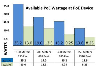
Results charted were calculated with a 20AWG center conductor and power sourcing equipment using IEEE 802.AF standard with starting voltage of 48 volts DC and IEEE 802.AT standard with starting voltage of 54 volts DC PoE Switches with internal power and current limits may change individual results.
