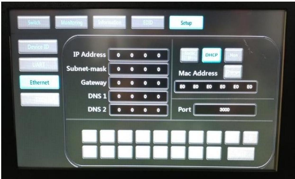
Press the Setup button to make other settings such as UART, Ethernet, and TEST Pattern.
