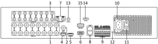
NOTE The rear panel of DS-8108HQHI-K8 provides 8 video input interfaces.
