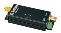
The FTD100Micro series supports optical transmission of 8-bit PCM coded video through one multimode or singlemode optical fiber. It is the smallest video transmitter/receiver pair among all OT Systems products. The transmitter only occupies limited space for easy installation within most camera housings.
