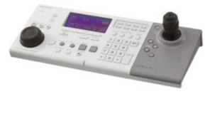
An optional RM-NS1000 System Controller - which connects to the NSR-1000 Series or a client PC via USB cable - allows the user to control multiple servers and cameras. A wide range of operations can be performed from this unit, including camera selection, Pan/ Tilt/Zoom (PTZ) with preset controls, snapshot capturing, video exporting, and event search and playback.
